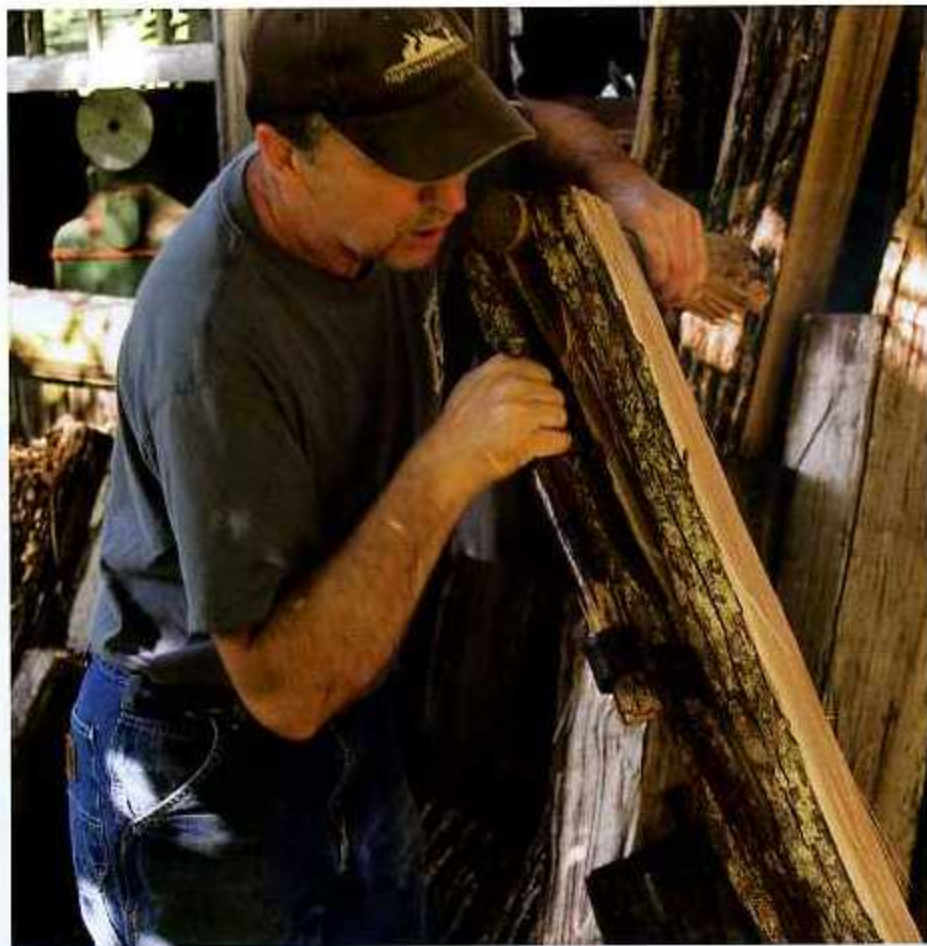
Curtis Buchanan uses a froe to rive out a chair back from a length of white oak.
