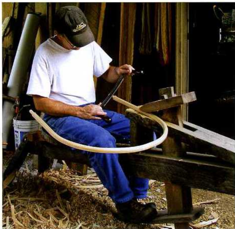
At the shaving horse, trimming a tenon on a loop-back chair.
